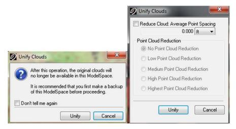
Figure 8 – Dialog boxes for which scanworlds are unified into one point cloud.
